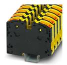
High-current terminal block, nom. voltage: 1000 V, nominal current: 125 A, number of connections: 2, number of positions: 1, connection method: PowerTurn connection, Rated cross section: 35 mm<sup>2</sup>, cross section: 2.5 mm<sup>2</sup> - 35 mm<sup>2</sup>, mounting type: NS 35/15, color: black/yellow
