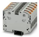
High-current terminal block, nom. voltage: 1000 V, nominal current: 125 A, number of connections: 2, connection method: PowerTurn connection, Rated cross section: 35 mm<sup>2</sup>, cross section: 2.5 mm<sup>2</sup> - 35 mm<sup>2</sup>, mounting type: NS 35/15, color: gray
