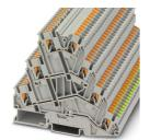
Motor terminal block, four-level, connection method: push-in connection, cross section: 0.14 mm<sup>2</sup> - 4 mm<sup>2</sup>, AWG: 26- 12, width: 5.2 mm, height: 91.1 mm, color: gray, mounting type: NS 35/7,5, NS 35/15
