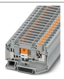
Test disconnect terminal block, connection method: Push-in connection, Screw connection, cross section: 0.5 mm<sup>2</sup> - 10 mm<sup>2</sup>, AWG: 20 - 10, width: 8.2 mm, color: gray, mounting: NS 35/7,5, NS 35/15
