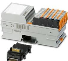
Axioline F, Function module, Counter inputs: 2, Incremental encoder inputs: 2, Symmetrical and asymmetrical encoders, Digital inputs: 8, 24 V DC, Digital outputs: 2, 24 V DC, transmission speed in the local bus: 100 Mbps, degree of protection: IP20, including bus base module and Axioline F connectors
