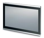
Touch panel with 47.0 cm / 18.5" TFT-display (Projective-capacitive (PCAP)), 1366 x 768 pixel(s) (WXGA), 65536 colors, Arm® Cortex®-A8, 1000 MHz, 2x USB host 2.0, 1 x Ethernet (10/100 Mbps), RJ45, Windows® Embedded Compact 7 and user software: Visu+. (bus system: without)
