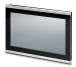
Touch panel with 30.7 cm/12.1" TFT-display (Projective-capacitive (PCAP)), 1280 x 800 pixel(s) (WXGA), 65536 colors, Arm® Cortex®-A8, 1000 MHz, 2x USB host 2.0, 1 x Ethernet (10/100 Mbps), RJ45, Windows® Embedded Compact 7 and user software: Visu+. (bus system: without)
