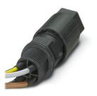
Panel feed-through, product family: QPD, connection method: Single wires/ IDC connection, number of positions: 3+PE, M20, Pin, 0.5 mm<sup>2</sup> ... 1.5 mm<sup>2</sup>, 690 V, 17.5 A, PA, black, with QUICKON nut, external cable diameter: 10 mm ... 13 mm, 1.5 mm<sup>2</sup>, cable length: 1 m
