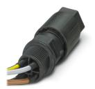
Panel feed-through, product family: QPD, connection method: Single wires/ IDC connection, number of positions: 3+PE, M20, Pin, 0.5 mm<sup>2</sup> ... 1.5 mm<sup>2</sup>, 690 V, 17.5 A, PA, black, with QUICKON nut, external cable diameter: 10 mm ... 13 mm, 1.5 mm<sup>2</sup>, cable length: 0.5 m
