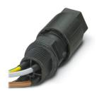
Panel feed-through, product family: QPD, connection method: Single wires/ IDC connection, number of positions: 3+PE, M20, Pin, 0.5 mm<sup>2</sup> ... 1.5 mm<sup>2</sup>, 690 V, 17.5 A, PA, black, with QUICKON nut, external cable diameter: 5 mm ... 9.5 mm, 1.5 mm<sup>2</sup>, cable length: 1 m
