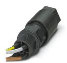
Panel feed-through, product family: QPD, connection method: Single wires/ IDC connection, number of positions: 3+PE, M20, Pin, 0.5 mm<sup>2</sup> ... 1.5 mm<sup>2</sup>, 690 V, 17.5 A, PA, black, with QUICKON nut, external cable diameter: 5 mm ... 9.5 mm, 1.5 mm<sup>2</sup>, cable length: 0.5 m
