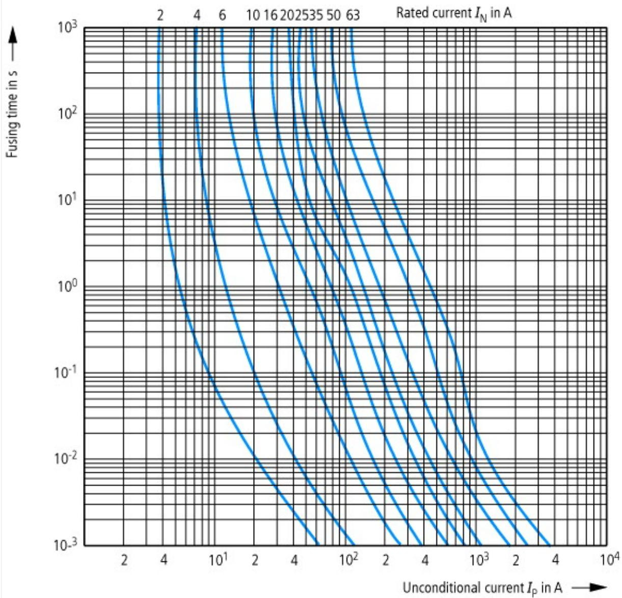
Time/current characteristic, D0 fuse links 2...63 A gG(gL)
