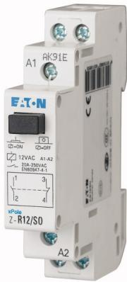
**Installation relay, 12VAC/50Hz, 1N/O+1N/C, 20A, 1HP**
