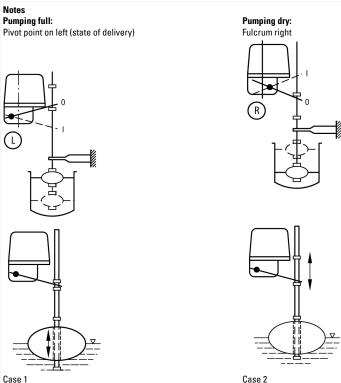
The actuation mechanism can either be connected to the float switch's actuation lever (configuration 1) or to the float (configuration 2). In configuration 1, the float drives the rod and the actuation lever. In configuration 2, the float and the rod drive the actuation lever. The latter configuration should especially be used in applications with sewage pumps.
