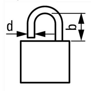
d = 4 - 8 mm  $b + d \leq 47 \text{ mm}$  d = 0.16 - 0.31 d = 4 - 8 mm d = 4 - 8 mm
