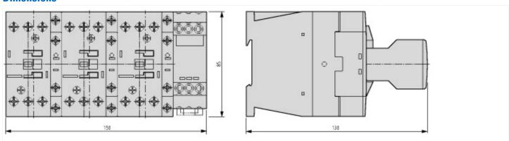
Basic unit with auxiliary contact module
