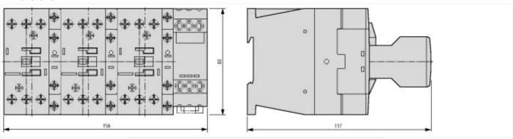
Basic unit with auxiliary contact module
