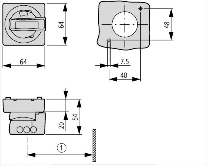
Mounting depth: 152 to 267 mm from the top edge of the top-hat rail to the front edge of the cabinet door/cover
