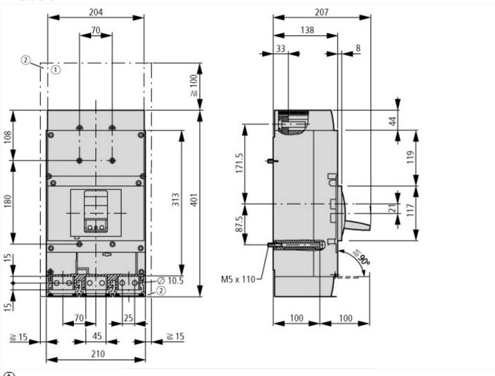
Blow out area, minimum clearance to adjacent parts Ui  $\leq$  690 V: 100 mm Ui  $\leq$  1500 V: 200 mm
