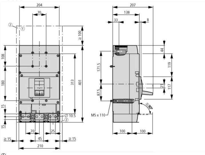
Blow out area, minimum clearance to adjacent parts Ui  $\leq$  690 V: 100 mm Ui  $\leq$  1500 V: 200 mm
