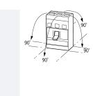
With residual-current release XFI: - NZM1, N1, NZM2, N2: vertical and 90° in all directions with plug-in adapter elements
