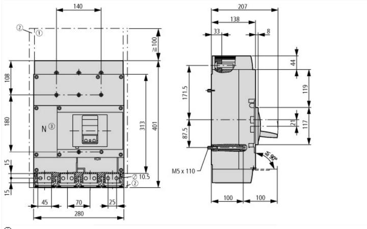
Blow out area, minimum clearance to adjacent parts: Ui  $\leq$  690 V: 100 mm Ui  $\leq$  1500 V: 200 mm
