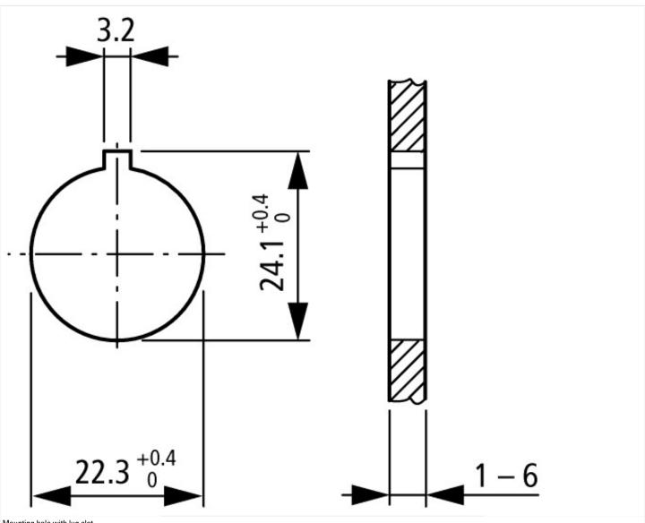
Mounting hole with lug slot
