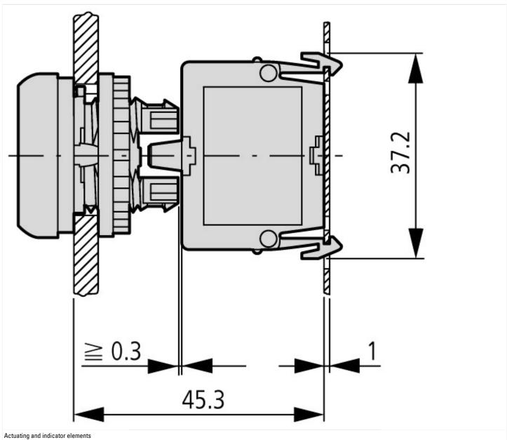
Actuating and indicator elements Base fixing
