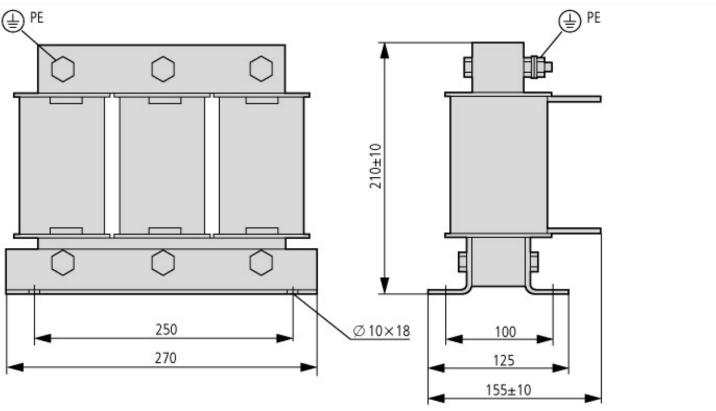
Height tolerance depends on gap The position of connection lugs U2-V2-W2 depends on the coil material and can deviate from the position illustrated here.
