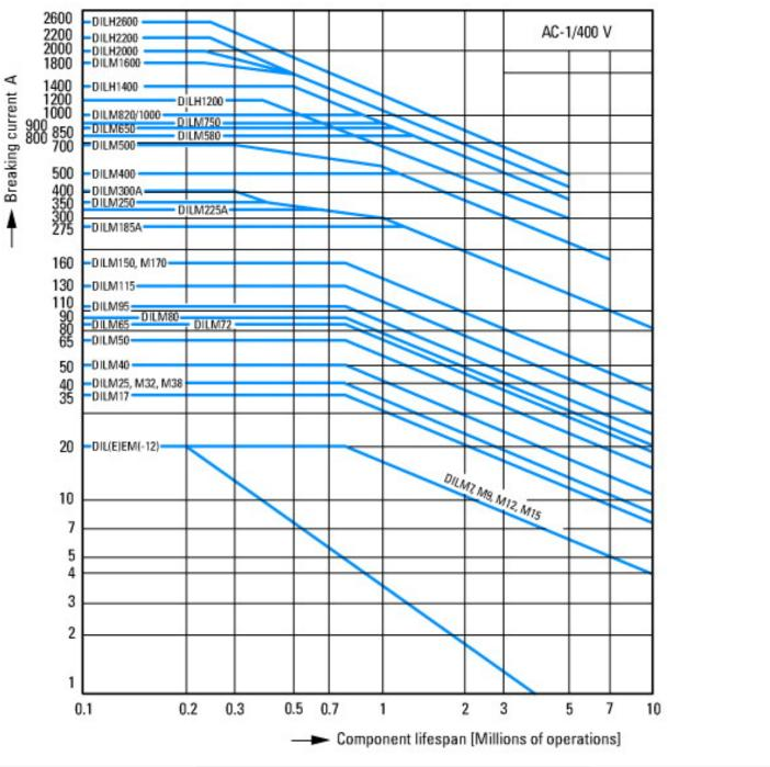
Switching conditions for 4 pole, non-motor loads Operating characteristics
