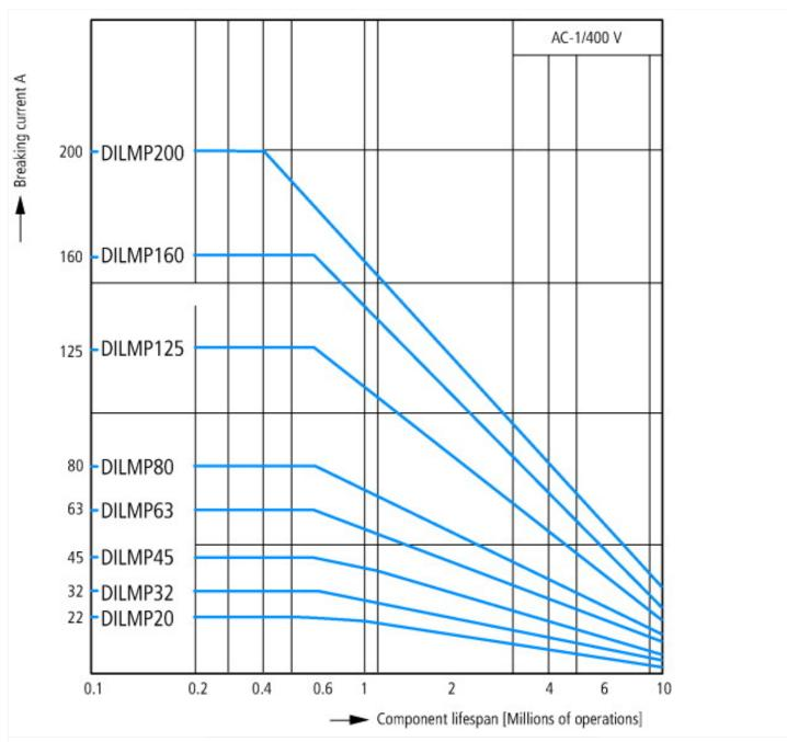
Switching conditions for 4 pole, non-motor loads Operating characteristics
