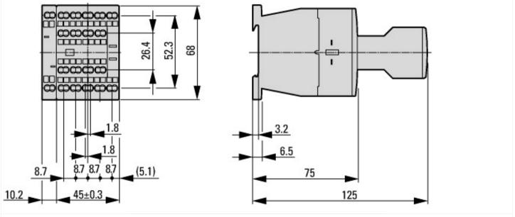
Contactor with auxiliary contact module
