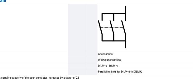
Instructions AC1 current carrying capacity of the open contactor increases by a factor of 2.5 Protected against accidental contact in accordance to VDE 0106 part 100
