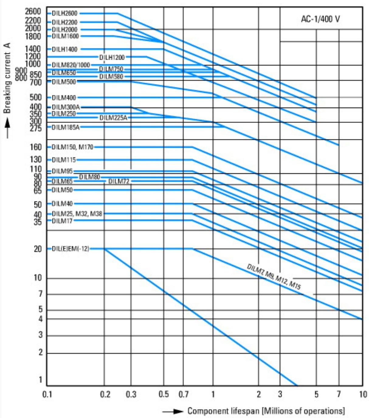
Switching conditions for 3 pole, non-motor loads
