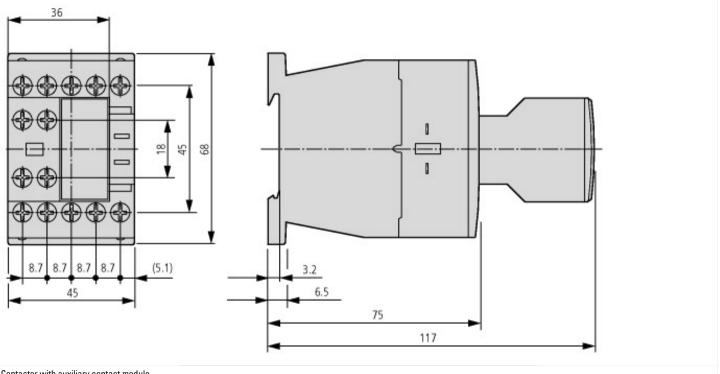
Contactor with auxiliary contact module
