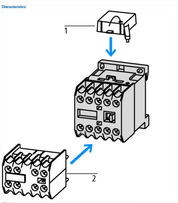
1: Suppressor 2: Auxiliary contact module
