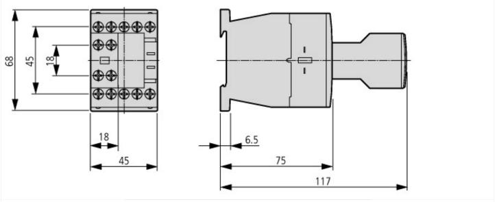
Contactor with auxiliary contact module
