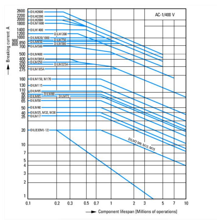
Switching duty for non-motor loads, 3-pole, 4-pole Operating characteristics
