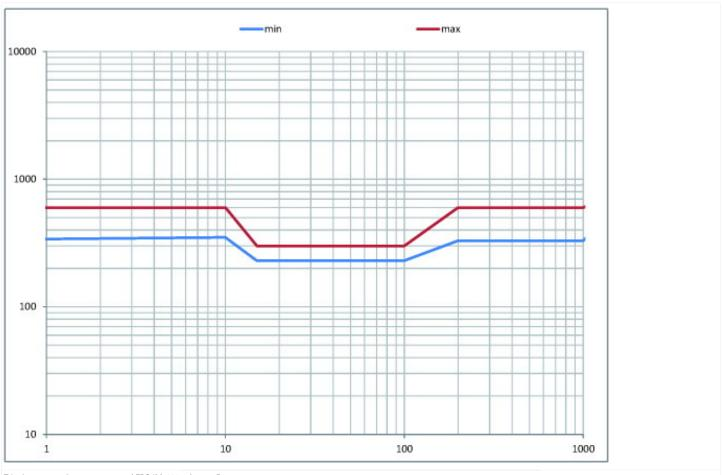
Tripping current frequency range: | FRCdM, 300 mA, type B
